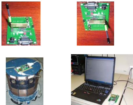
Transceiver 2(Robot site) Transceiver 1(PC site) Fig.4:Radio communication between the robot and PC
